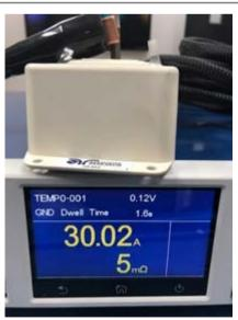
Remove the connection from the front panel and attach "HV", "Current" and "Return" on the backside of the instrument. Repeat the 30 Amp test to ensure the resistance is below 10 mOhms.
