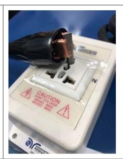
Connect the adapter box to the front panel "Current", "Sense +", and "HV" connections.
