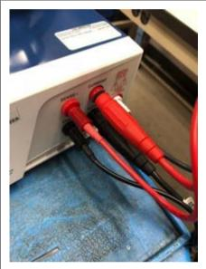
Setup a 30 Amp Ground Bond test for 5 seconds with rest of the test parameters set to default. A measurement of less than 10 mOhms indicates a successful test.
